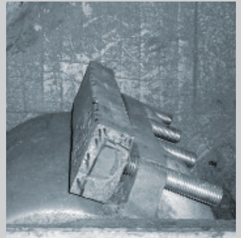
Glass recycling; impact crusher for crushing of ceramics
